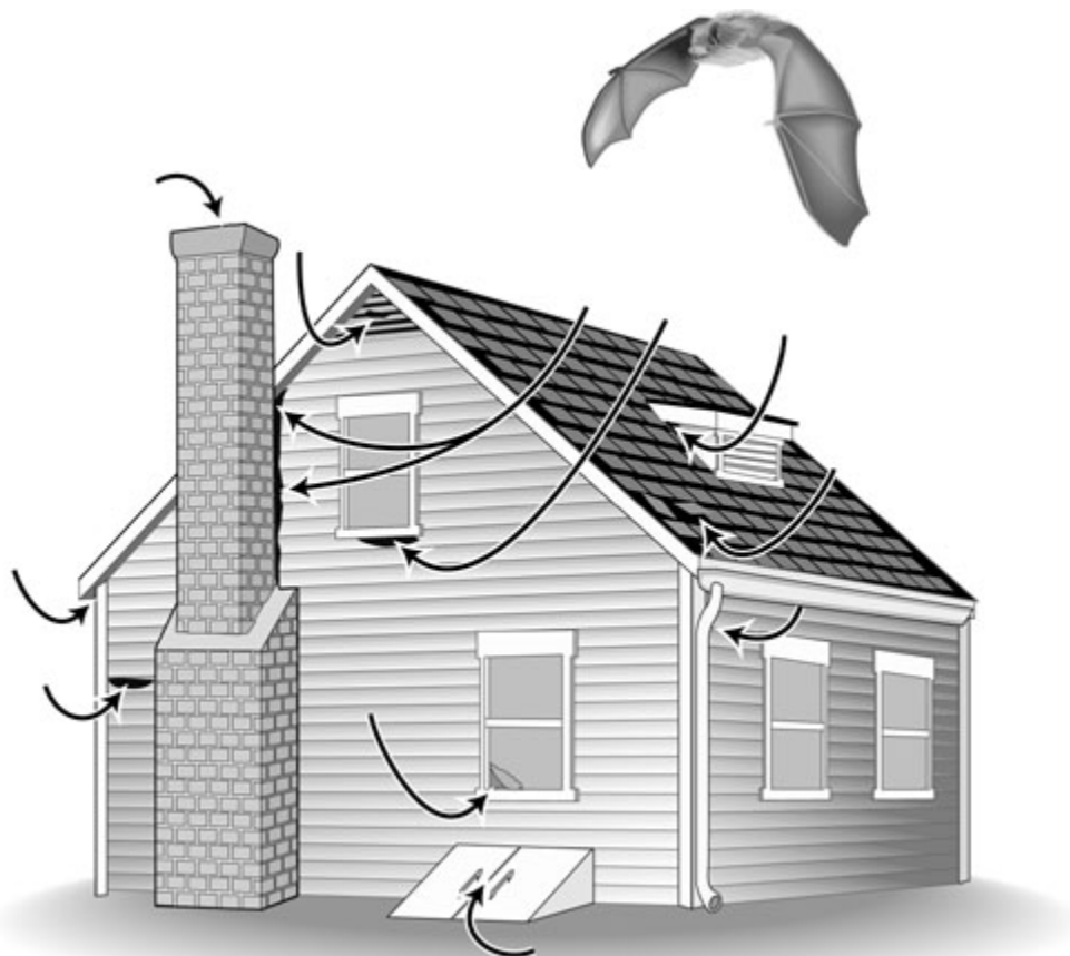
Common entry points on homes and buildings include corners, eaves and louvres.
